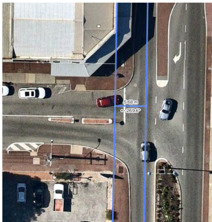
Figure 3: Minimum available sightline setback at intersection
